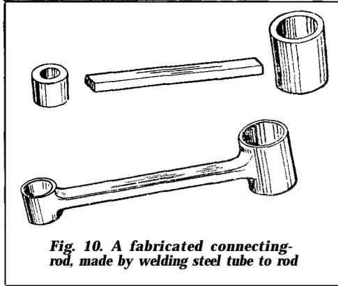
**Fig. 10. A fabricated connecting-rod, made by welding steel tube to rod**
