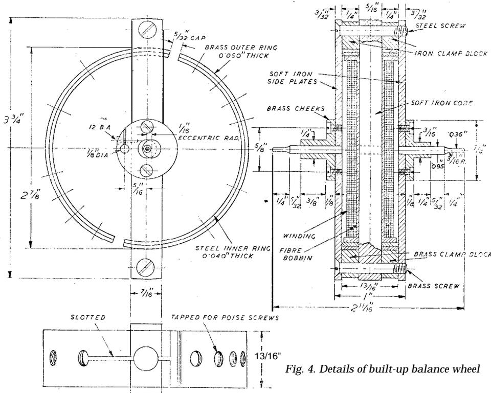
Fig. 4. Details of built-up balance wheel
