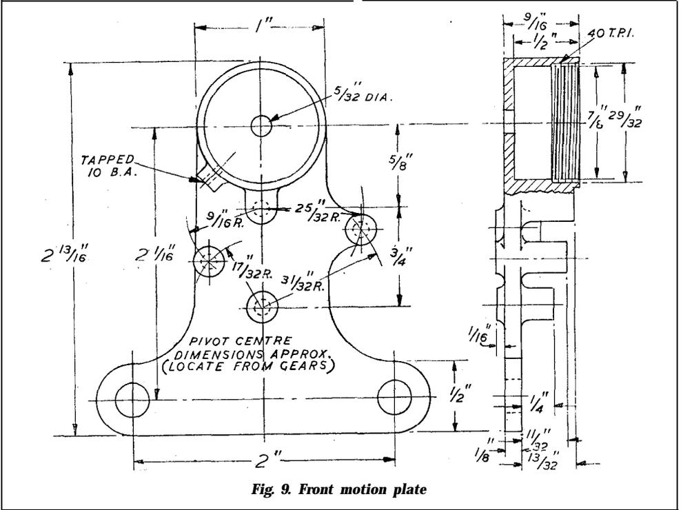
Fig. 9. Front motion plate
