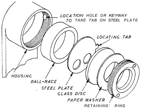
Below-Fig. 11. Exploded view of bearing assembly
