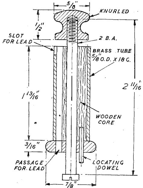
Fig. 21 Supporting pillars, 2 off (one only drilled and located to form lead conduit)
