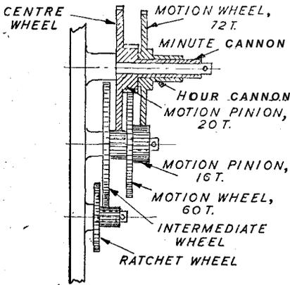
Fig. 20. Diagrammatic side view of wheel train
