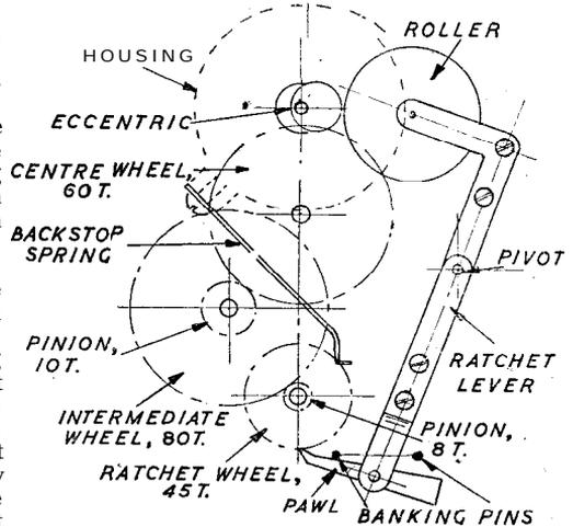
Fig. 19. Arrangement of ratchet gear and main wheel train
