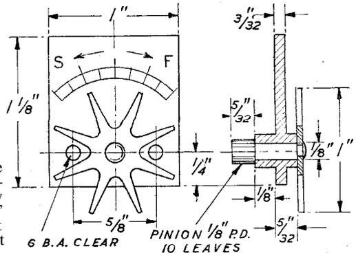
Fig. 15. Regulator pinion, star wheel and rating plate
